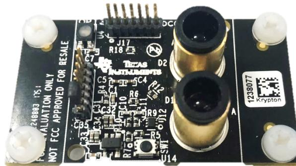
**Figure 1. OPT3101EVM Printed-Circuit Board**
