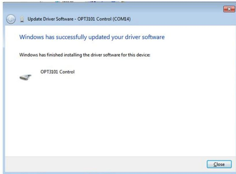
14. Now repeat this process (steps 1 to 13) for *OPT3101 Data*. All steps are the same except for step 2 and step 11. In step 2 make sure to right click *OPT3101 Data* instead of *OPT3101 Control*. Likewise, on step 11 make sure to select *OPT3101 Data* instead of *OPT3101 Control* when installing the driver as the following figure shows.
