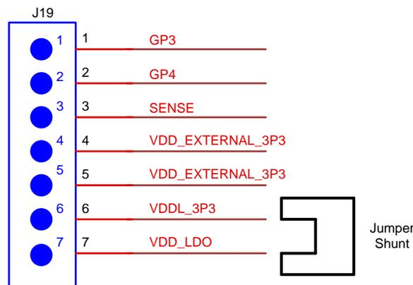
Figure 6. J19 Header With Power-On Jumper Shown
