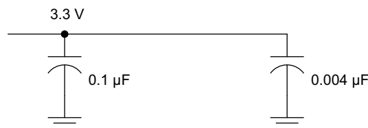
图 17. Recommended M-LVDS Bypass Capacitor Layout
