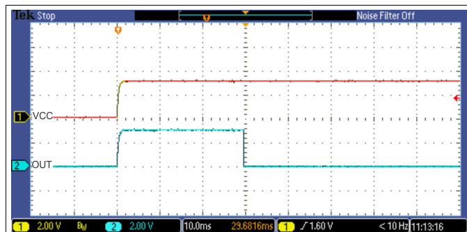
Figure 14. TMP303A Power-On Response, T_A Less Than 60°C
