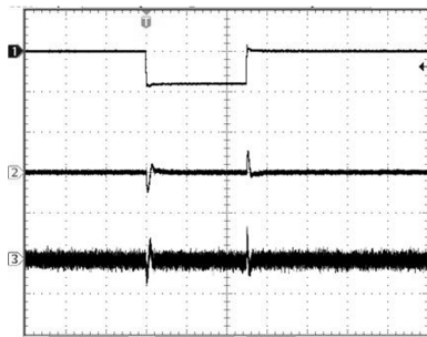
Channel 1: V_{IN} (500mV/div) Time Base (400µs/div) Channel 2: V_{OUT} (500mV/div) L = 22\ \mu\text{H} Channel 3: I_{LED} (500µA/div) I_{LED} = 19\ \text{mA} V_{IN} From 3.6 V To 3.2 V
