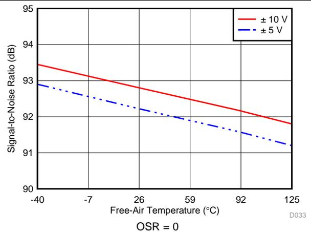
Figure 37. SNR vs Temperature for Different Input Ranges
