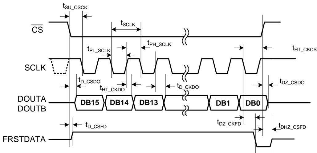
Figure 5. Serial Data Read Operation Timing Diagram
