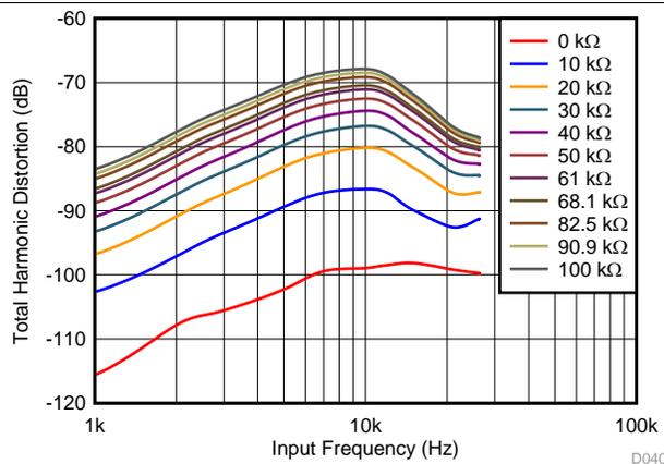
Figure 44. THD vs Input Frequency for Different Source Impedances ( $\pm 10\text{ V}$ )
