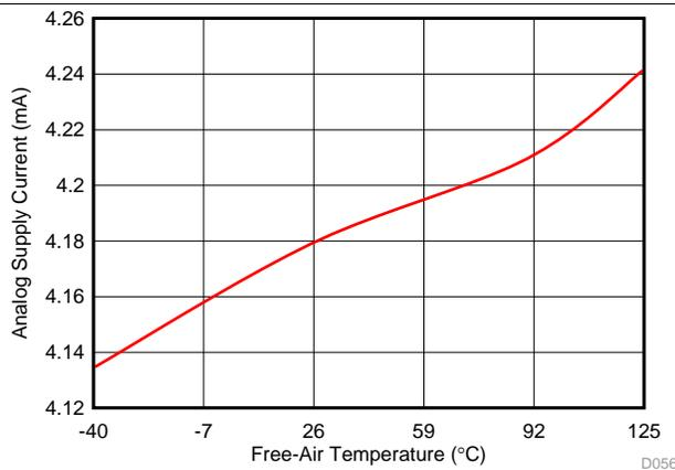
**Figure 50. Analog Supply Current vs Temperature (Standby)**
