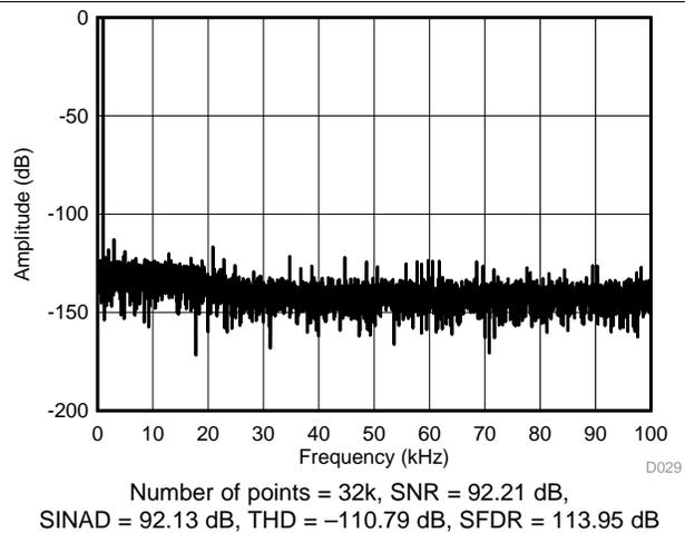
Figure 33. Typical FFT Plot ( $\pm 5\text{ V}$ )
