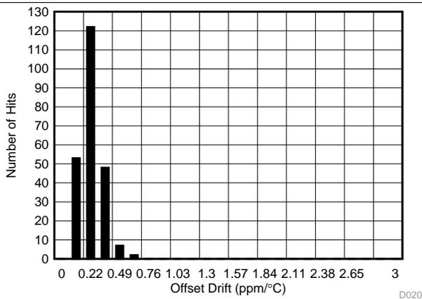
Figure 24. Offset Drift Histogram Distribution ( $\pm 5\text{ V}$ )
