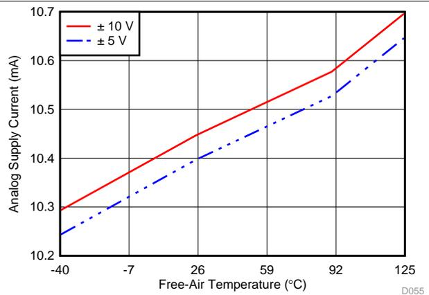
**Figure 49. Analog Supply Current (Static) vs Temperature (Sampling)**
