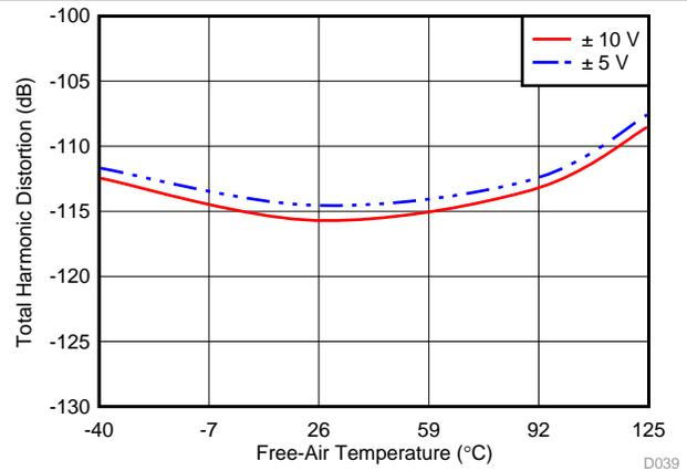
Figure 43. THD vs Temperature for Different Input Ranges
