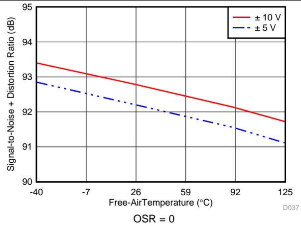
Figure 41. SINAD vs Temperature for Different Input Ranges
