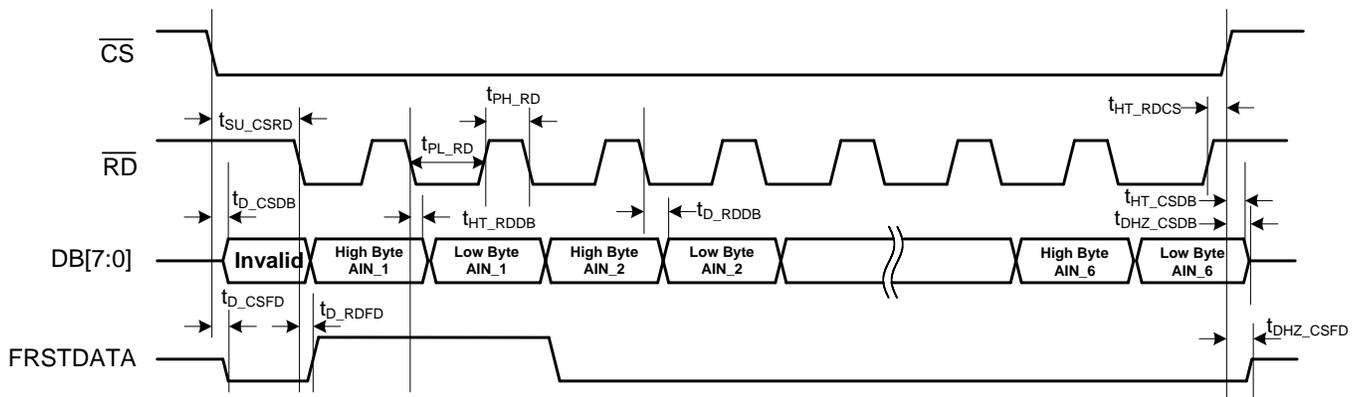
Figure 6. Byte Mode Data Read Operation Timing Diagram
