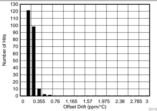
Figure 22. Offset Drift Histogram Distribution ( $\pm 10\text{ V}$ )
