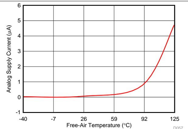
**Figure 51. Analog Supply Current vs Temperature (Shutdown)**
