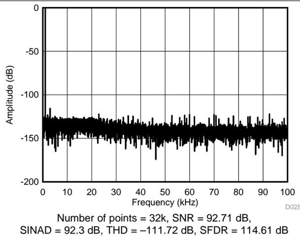
Figure 32. Typical FFT Plot ( $\pm 10\text{ V}$ )
