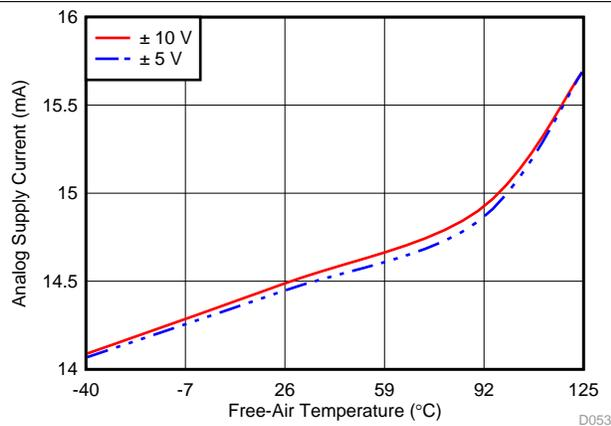
**Figure 48. Analog Supply Current (Operational) vs Temperature**
