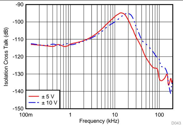
**Figure 47. Isolation Crosstalk vs Noise Frequency (Saturated Inputs)**
