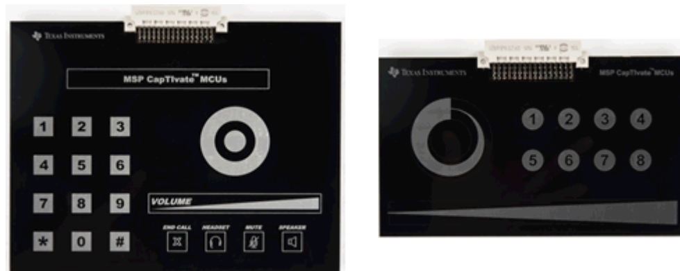
图 10-6. CAPTIVATE-PHONE and CAPTIVATE-BSWP Panels
