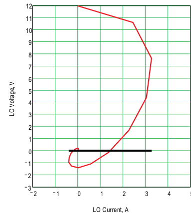
Figure 25. Turnoff Voltage and Current Switching Diagram
