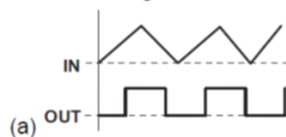
Figure 7. Schmitt Trigger Curves
