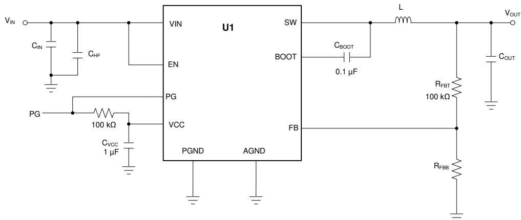
图 17. Circuit for Application Curves
