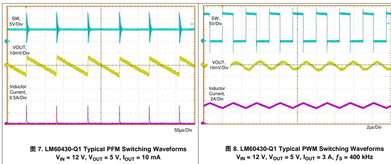
图 7. LM60430-Q1 Typical PFM Switching Waveforms
