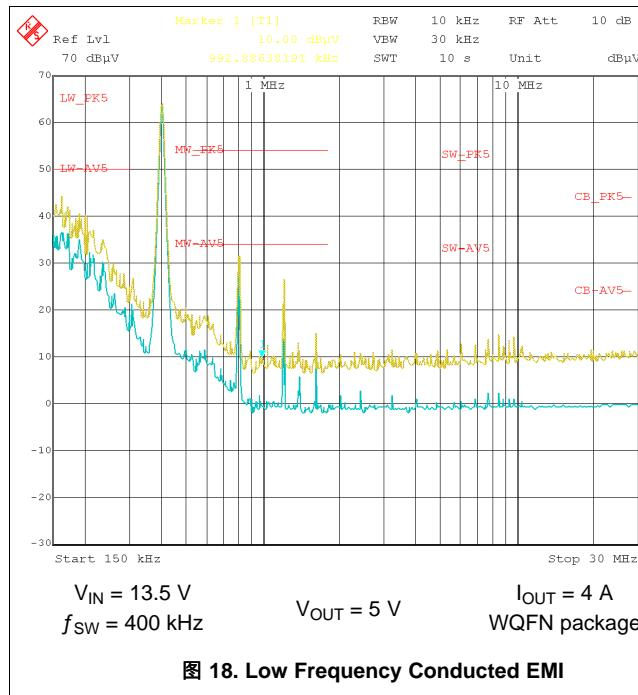
图 18. Low Frequency Conducted EMI
