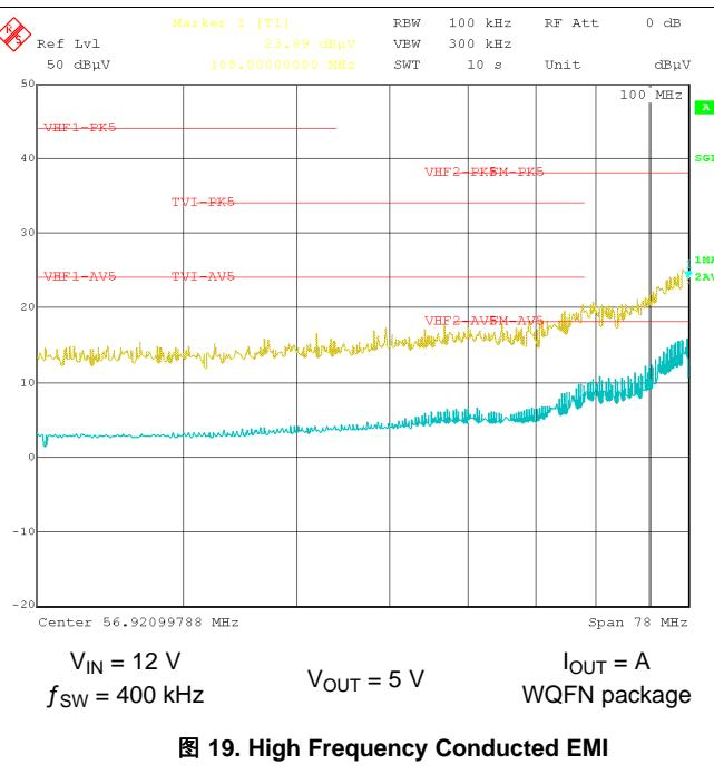
图 19. High Frequency Conducted EMI
