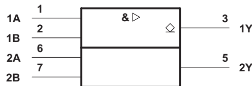
Figure 10. SNx5451B Logic Symbol
