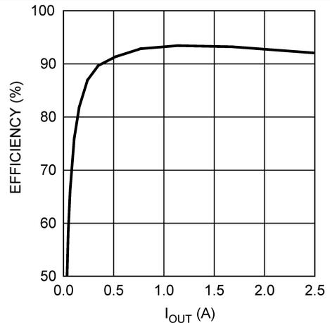
$V_{IN} = 5\text{ V}$        $V_{OUT} = 2.5\text{ V}$        $F_{SW} = 379\text{ kHz}$
