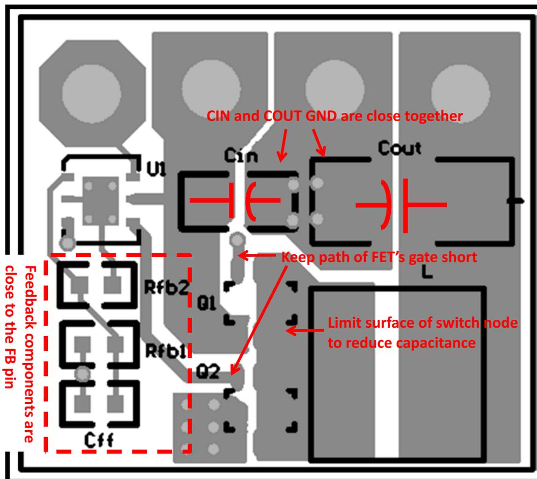
Figure 26. LM1771 Layout Example (Top)
