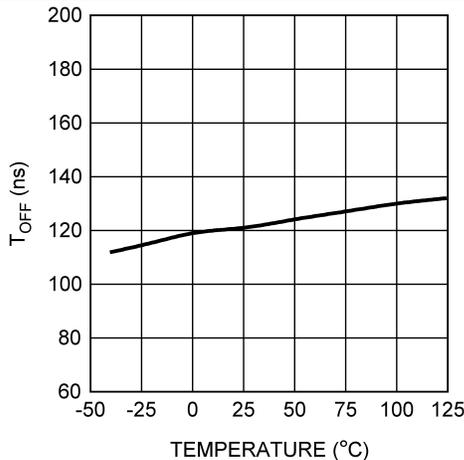
Figure 9. T<sub>OFF</sub> vs Temperature (LM1771U)
