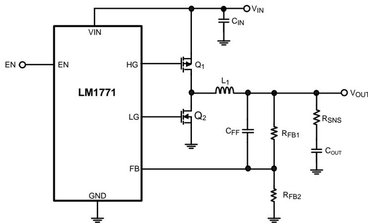
Figure 24. Example Circuit Schematic, 5 V<sub>IN</sub> to 1.8 V<sub>OUT</sub>
