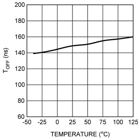
Figure 7. T<sub>OFF</sub> vs Temperature (LM1771S)
