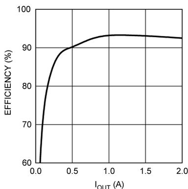
Figure 23. Typical Efficiency 5 V<sub>IN</sub> to 2.5 V<sub>OUT</sub>
