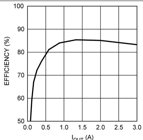
$V_{IN} = 5\text{ V}$        $V_{OUT} = 1.2\text{ V}$        $F_{SW} = 727\text{ kHz}$
