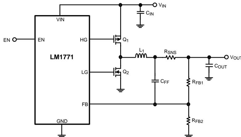
Figure 20. LM1771 With an External ESR Resistor ( $R_{SNS}$ )
