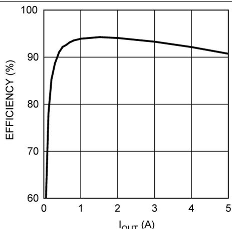
$V_{IN} = 5\text{ V}$        $V_{OUT} = 3.3\text{ V}$        $F_{SW} = 500\text{ kHz}$
