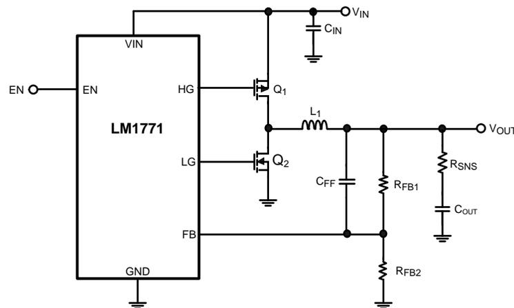
**Figure 25. Example Circuit Schematic, 5 V<sub>IN</sub> to 3.3 V<sub>OUT</sub>**
