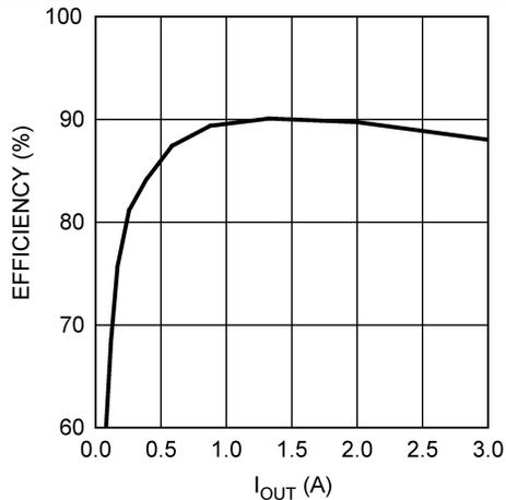
$V_{IN} = 5\text{ V}$        $V_{OUT} = 1.8\text{ V}$        $F_{SW} = 545\text{ kHz}$
