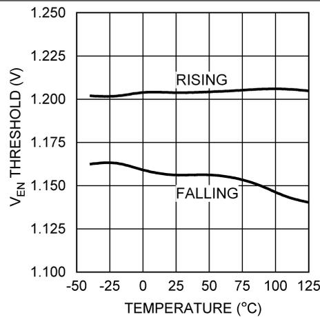
Figure 11. V<sub>EN</sub> Threshold vs Temperature
