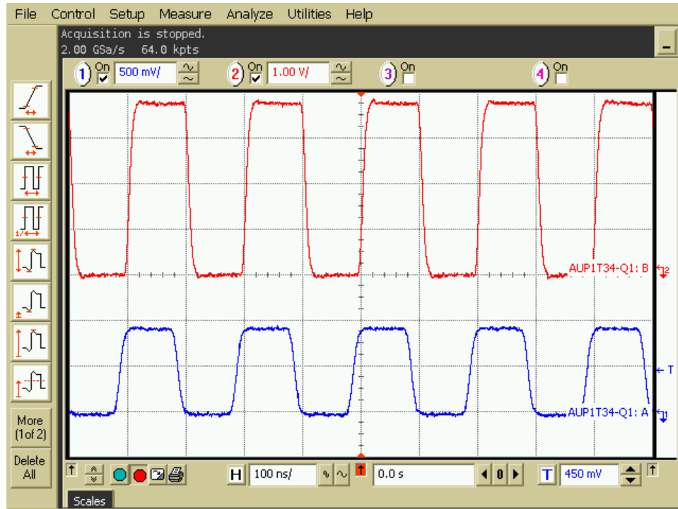
Figure 5. 10 MHz Up Translation (0.9 V to 3.6 V)
