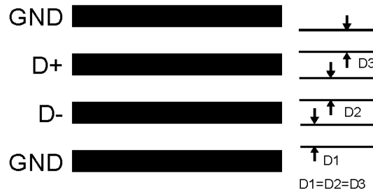
Figure 21. Ideal Diode Trace Layout
