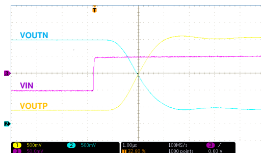
图 8-4. Step Response of the AMC1302
