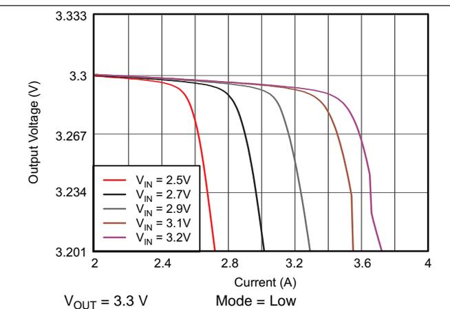
图 54. TPS61282A DC Output Voltage vs Output Current
