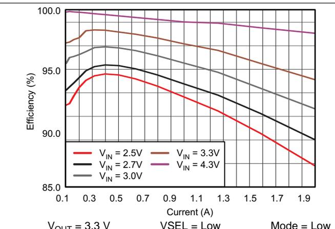
图 50. TPS61282A Efficiency vs Output Current
