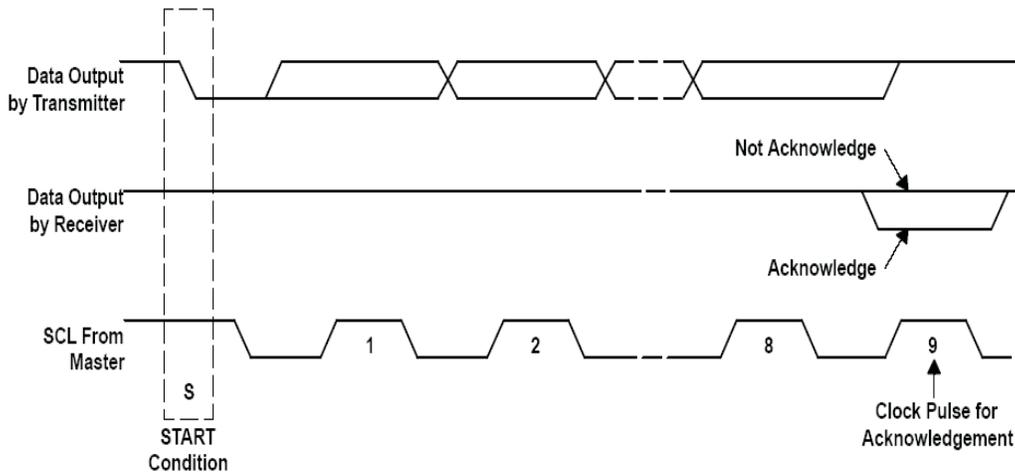
图 22. Acknowledge on the I<sup>2</sup>C Bus
