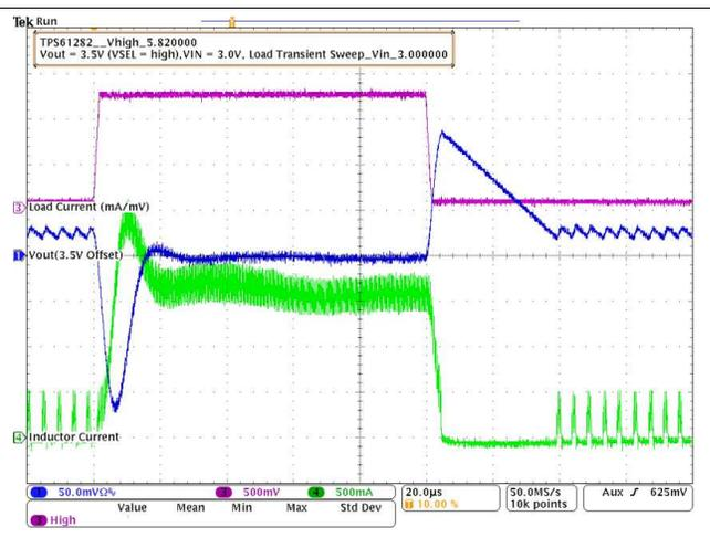
图 64. TPS61282A Load Transient Response In PFM/PWM Operation
