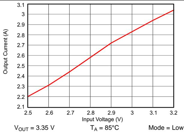
图 39. TPS61281A Maximum Output Current vs Input Voltage
