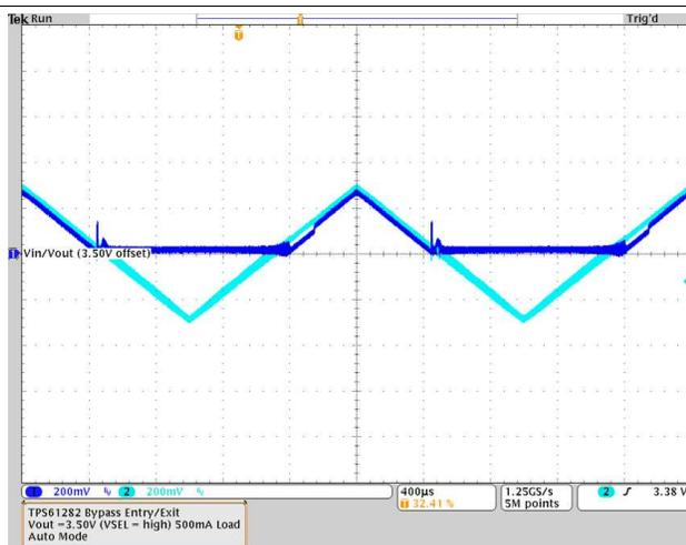
图 59. Boost to Pass-Through Mode Exit / Entry
