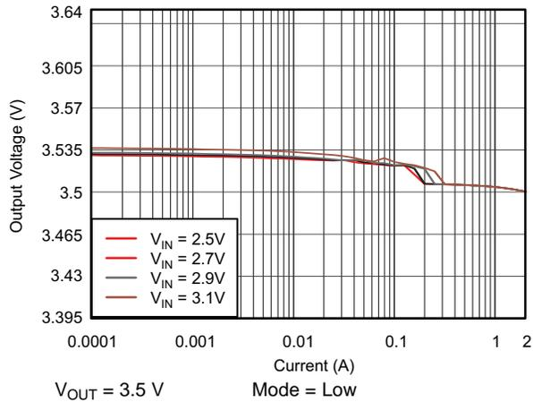
图 55. TPS61282A DC Output Voltage vs Output Current
