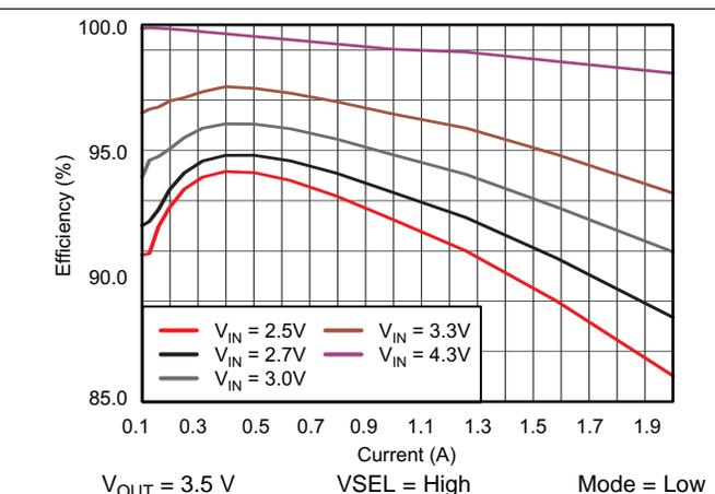
图 52. TPS61282A Efficiency vs Output Current
