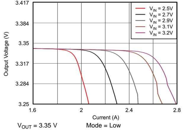
图 36. TPS61281A DC Output Voltage vs Output Current
