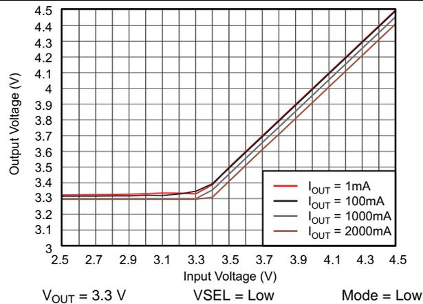
图 57. TPS61282A DC Output Voltage vs Input Voltage
