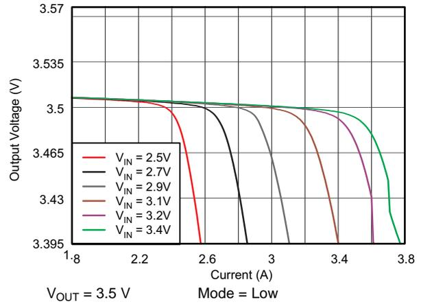
图 56. TPS61282A DC Output Voltage vs Output Current
