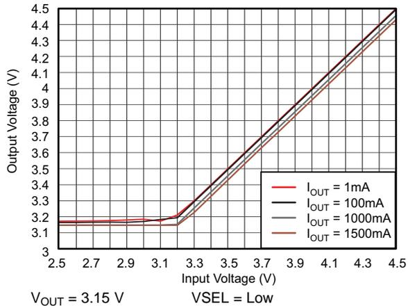
图 37. TPS61281A DC Output Voltage vs Input Voltage
