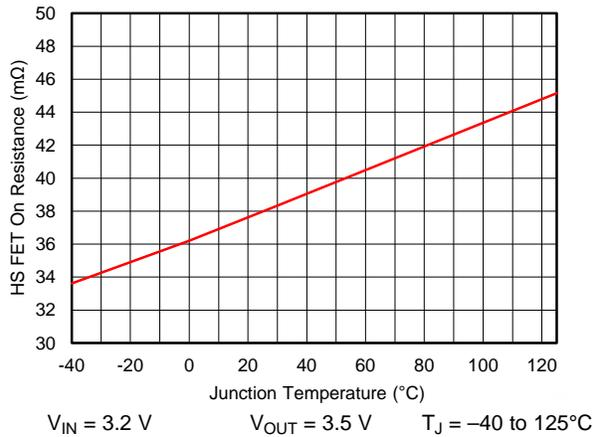
图 3. High side  $R_{ds(on)}$  vs Junction Temperature
