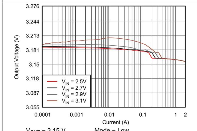
图 33. TPS61281A DC Output Voltage vs Output Current
