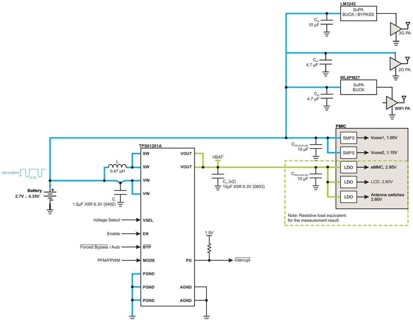
图 28. TPS61281A Application Circuit with 1500mA Output Current
