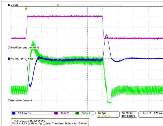
图 63. TPS61282A Load Transient Response In PWM Operation
