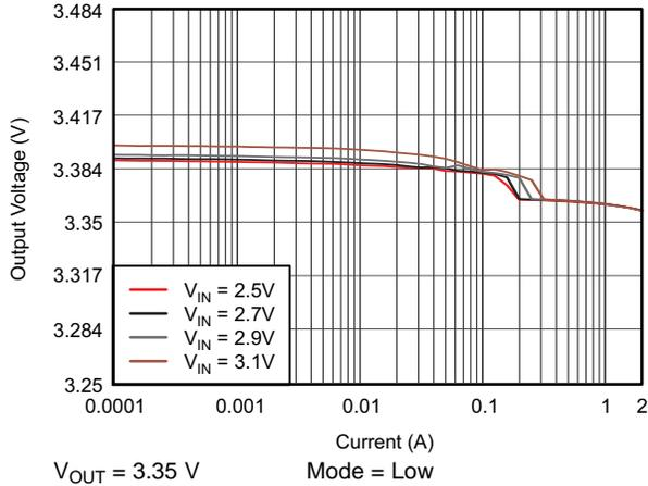
图 35. TPS61281A DC Output Voltage vs Output Current
