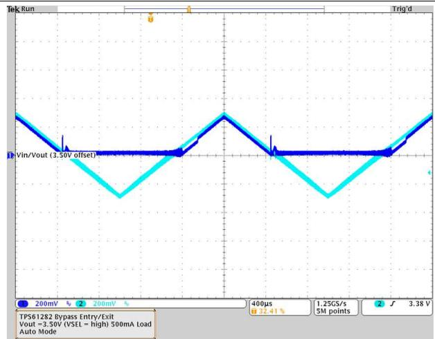
图 40. Boost to Pass-Through Mode Exit / Entry
