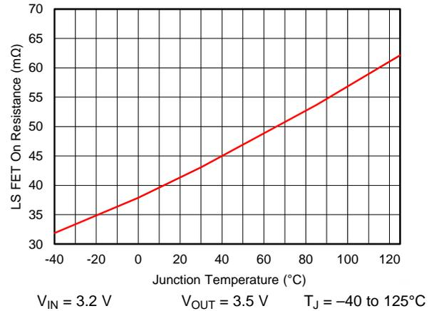
图 4. Low side  $R_{ds(on)}$  vs Junction Temperature
