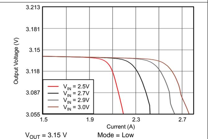
图 34. TPS61281A DC Output Voltage vs Output Current
