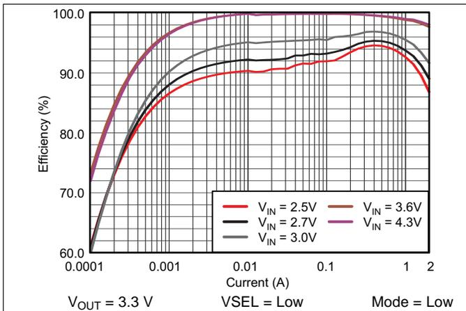
图 49. TPS61282A Efficiency vs Output Current
