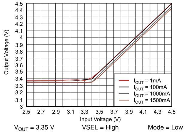
图 38. TPS61281A DC Output Voltage vs Input Voltage
