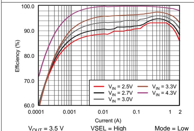
图 51. TPS61282A Efficiency vs Output Current
