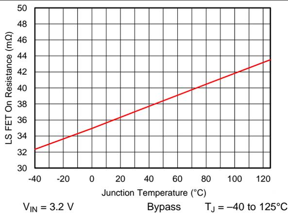
图 5. Bypass FET  $R_{ds(on)}$  vs Junction Temperature
