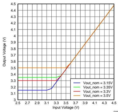
**图 18. DC Output Voltage vs. Input Voltage**
