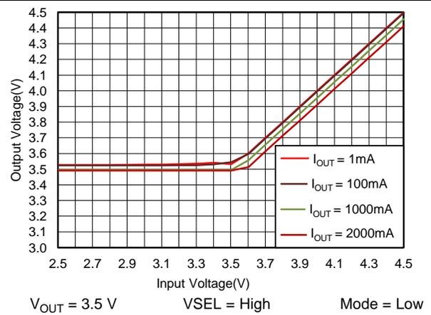
图 58. TPS61282A DC Output Voltage vs Input Voltage
