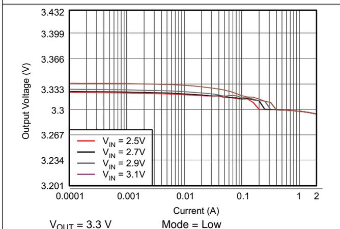
图 53. TPS61282A DC Output Voltage vs Output Current
