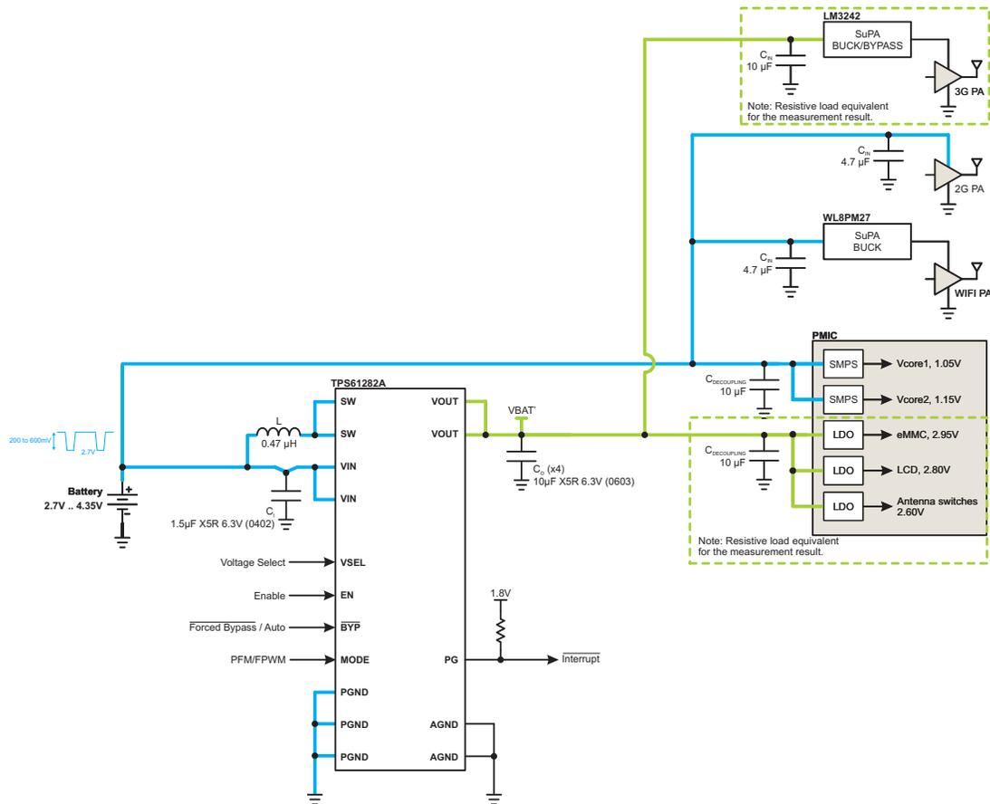
图 48. TPS61282A Application Circuit with 2000 mA Output Current
