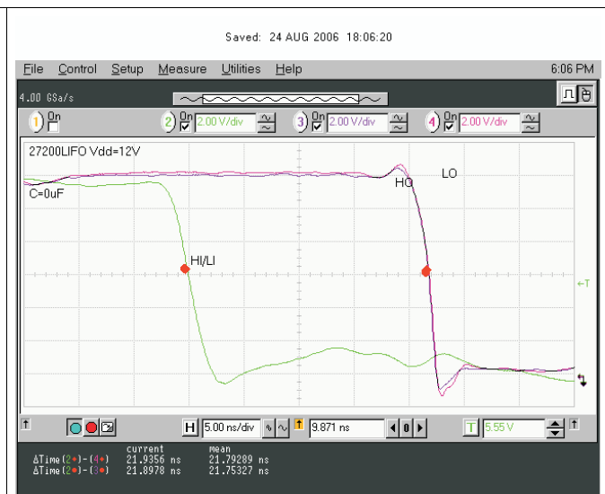
Figure 26. V_{LO} and V_{HO} Falling Edge Delay Matching
