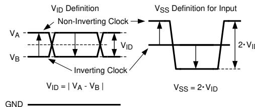
**Figure 8. Two Different Definitions for Differential Input Signals**
