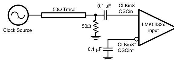
**Figure 27. CLKinX and OSCin Single-Ended Termination**
