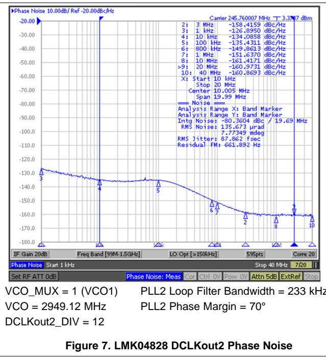
VCO\_MUX = 1 (VCO1) PLL2 Loop Filter Bandwidth = 233 kHz
