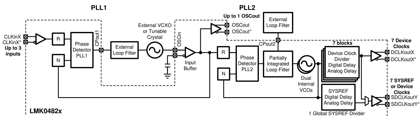
**Figure 18. Simplified Functional Block Diagram for Dual-Loop Mode**
