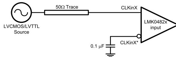
**Figure 28. DC-Coupled LVCMS/LVTTL Reference Clock**
