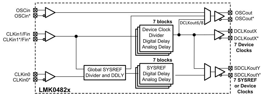
**Figure 23. Simplified Functional Block Diagram for Distribution Mode**
