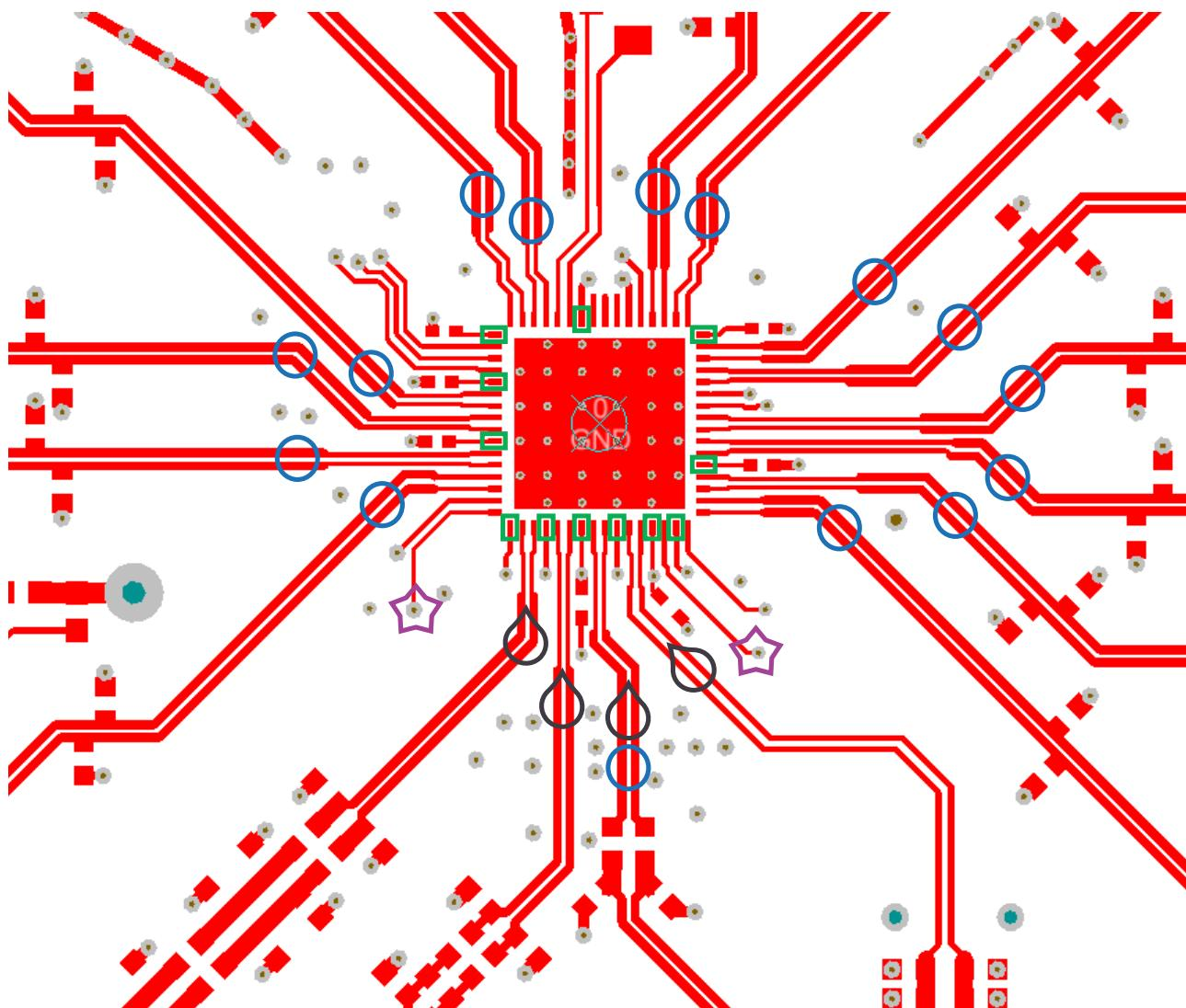
CLKin and OSCin path – if differential input (preferred) route traces tightly coupled. If single ended, have at least 3 trace width (of CLKin/OSCin trace) separation from other RF traces.
