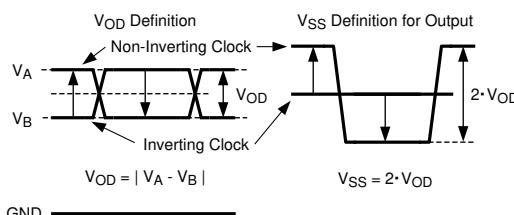
**Figure 9. Two Different Definitions for Differential Output Signals**
