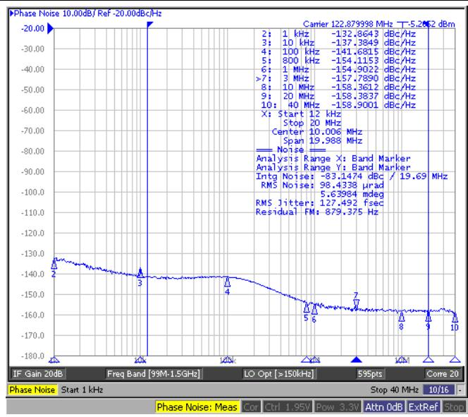
**Figure 37. SDCLKout11, 122.88 MHz, LVDS
