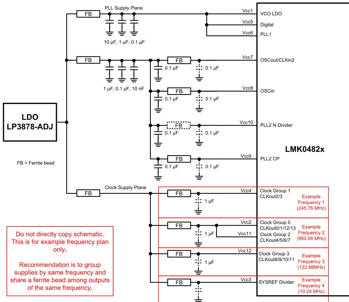
**Figure 41. Example Application - Power System Schematic**
