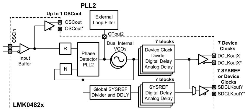
**Figure 21. Simplified Functional Block Diagram for Single-Loop Mode**
