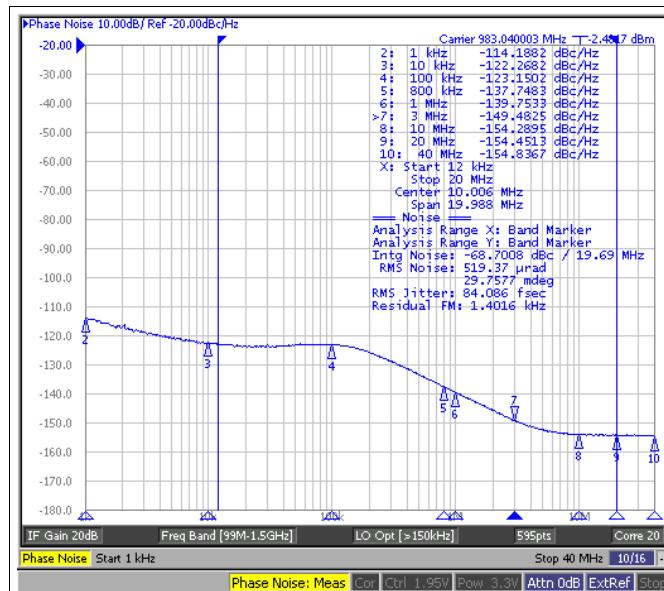
**Figure 34. DCLKout4, 983.04-MHz
