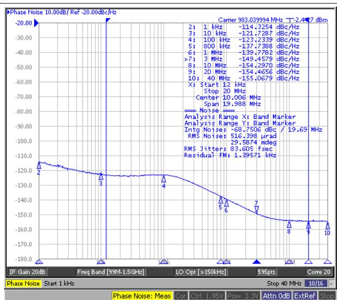
**Figure 35. DCLKout6, 983.04-MHz
