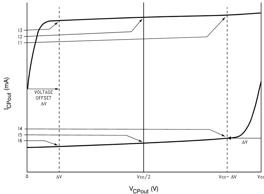
I1 = Charge Pump Sink Current at  $V_{CPOut} = V_{CC} - \Delta V$
