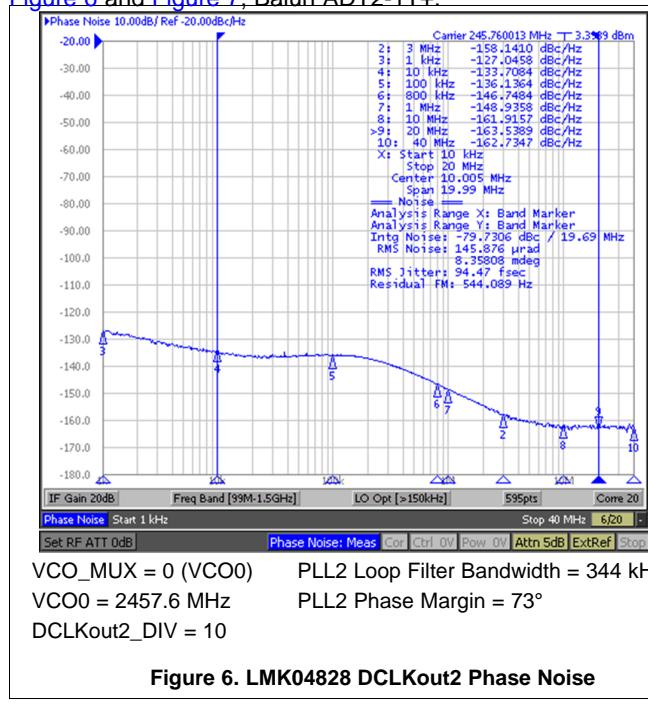
VCO\_MUX = 0 (VCO0) PLL2 Loop Filter Bandwidth = 344 kHz
