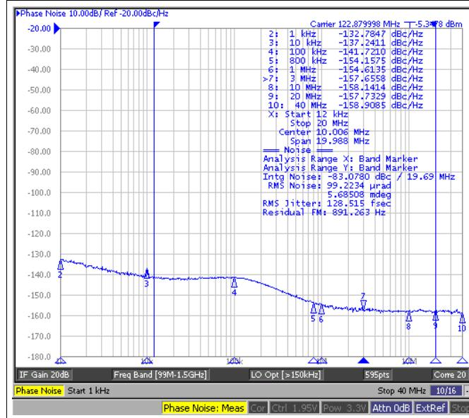
**Figure 36. DCLKout10, 122.88 MHz, LVDS
