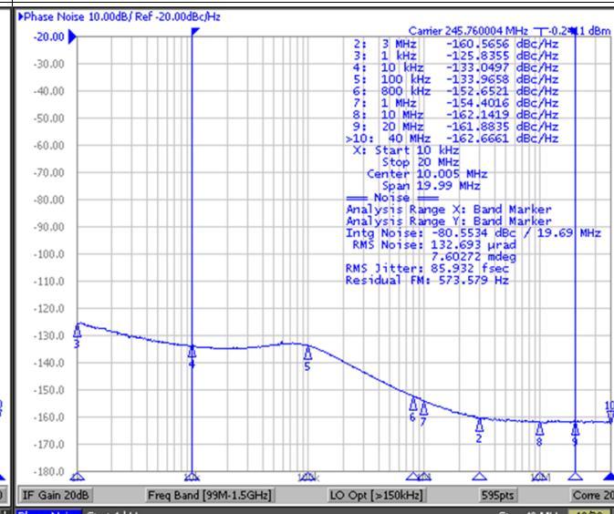
**Figure 4. LMK04826 DCLKout2 Phase Noise**
