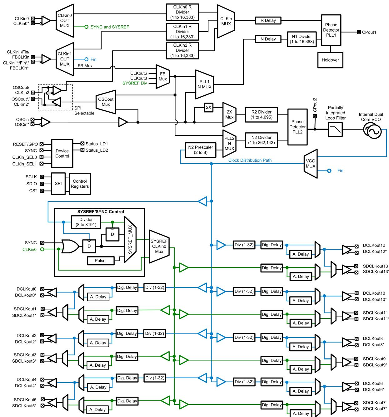
**Figure 11. Detailed LMK04826 and LMK04828 Block Diagram**
