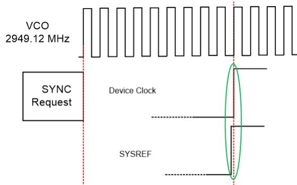
**Figure 16. SYSREF to Device Clock Timing Alignment**
