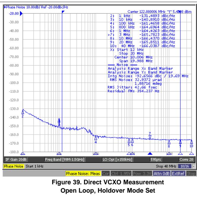
Figure 39. Direct VCXO Measurement
