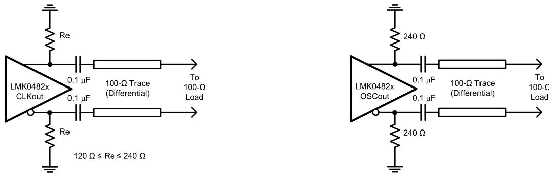
**Figure 29. LVPECL Biasing for CLKout and OSCout**
