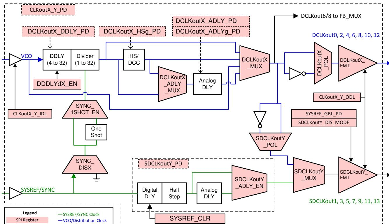
**Figure 12. Device and SYSREF Clock Output Block**
