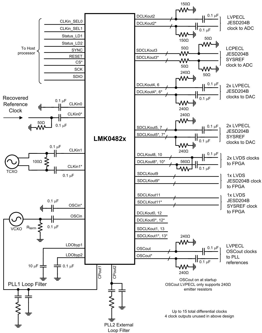
**Figure 40. Example Application - System Schematic Except for Power**
