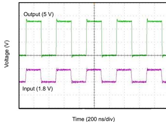
**Figure 4. Translation Up (1.8 V to 5 V) at 2.5 MHz**
