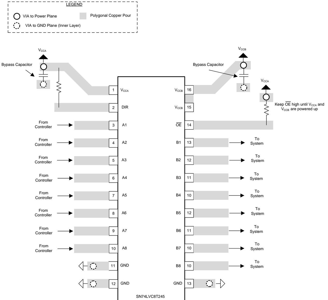
**Figure 5. SN74LVC8T245-EP Layout**
