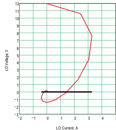
Figure 25. Turnoff Voltage and Current Switching Diagram
