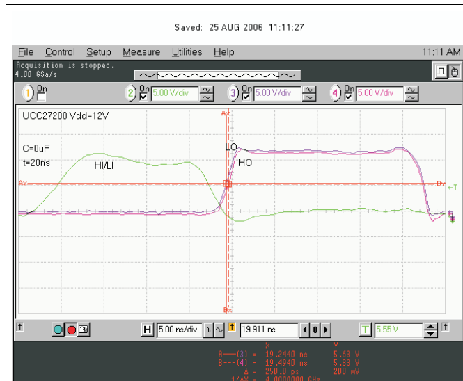
Figure 32. 20-ns Input Pulse Delay Matching
