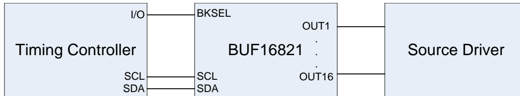
Figure 20. Gamma Control Block Diagram
