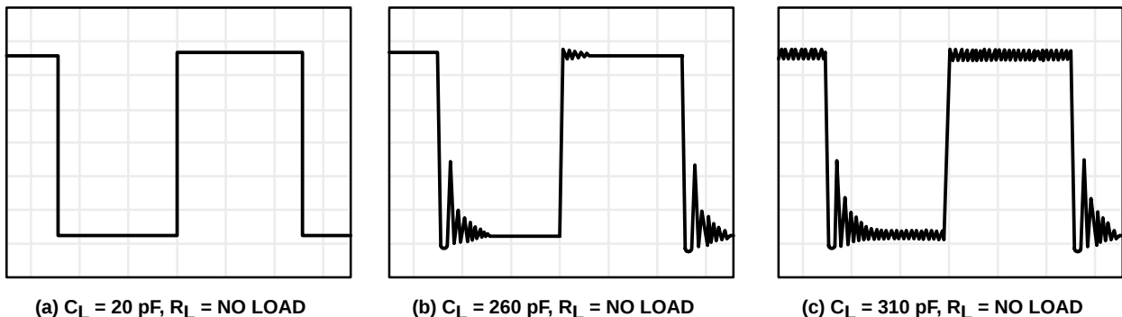
Figure 112. Effect of Capacitive Loads in Low-Bias Mode
