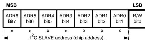
Figure 50. Address and Read/Write Bit
