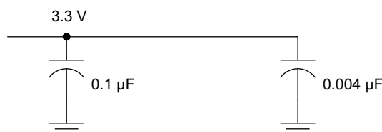
图 18. Recommended M-LVDS Bypass Capacitor Layout
