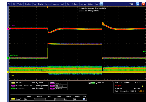
Figure 23. Transient Response Peak-to-Peak
