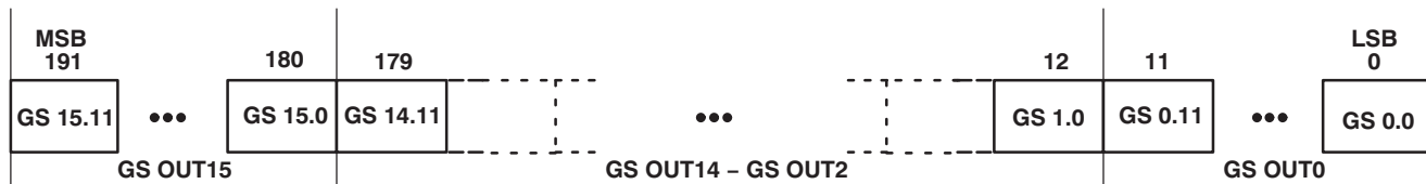
Figure 19. Grayscale Data Packet Format
