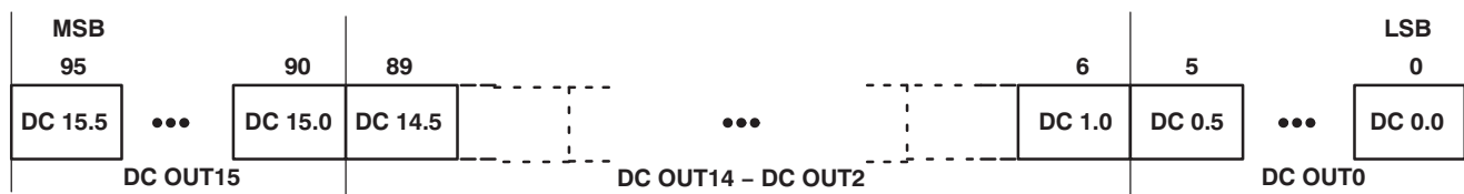
Figure 15. Dot Correction Data Packet Format
