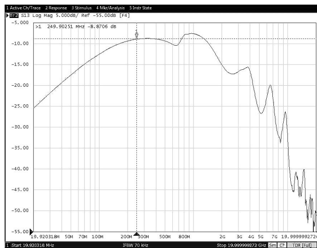
图 8-30. Off-State Data-Switch Isolation vs Frequency (TPS25830A-Q1)
