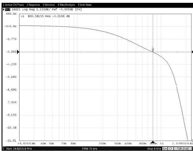
图 8-29. Data Transmission Characteristics vs Frequency (TPS25830A-Q1)
