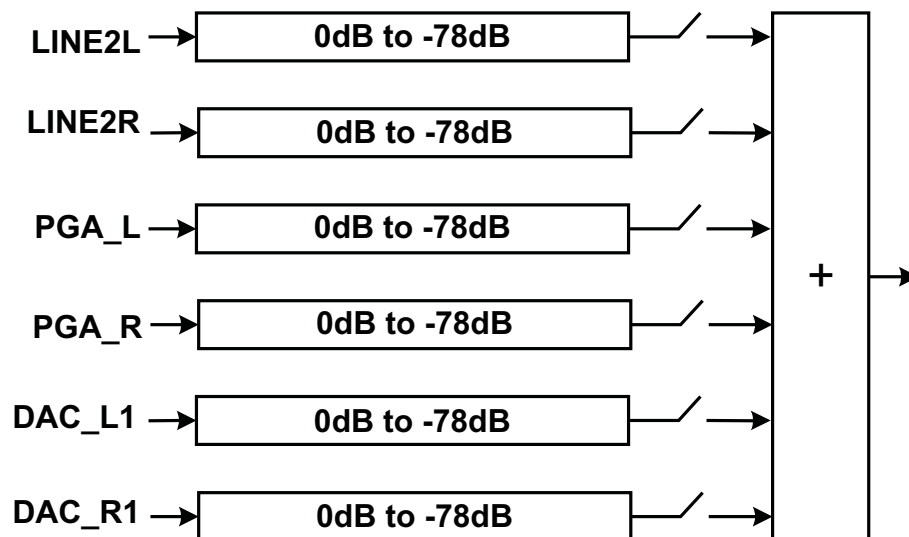
Figure 34. Detail of the Volume Control and Mixing Function Shown in Figure 26 and Figure 16
