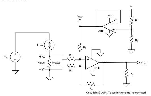
Figure 21. Bidirectional Current-Sensing Schematic
