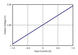
Figure 22. Bidirectional Current-Sensing Circuit Performance:
