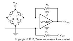
Figure 23. Single Operational Amplifier Bridge Amplifier Schematic
