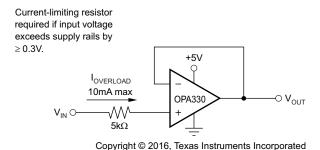
Figure 18. Input Current Protection
