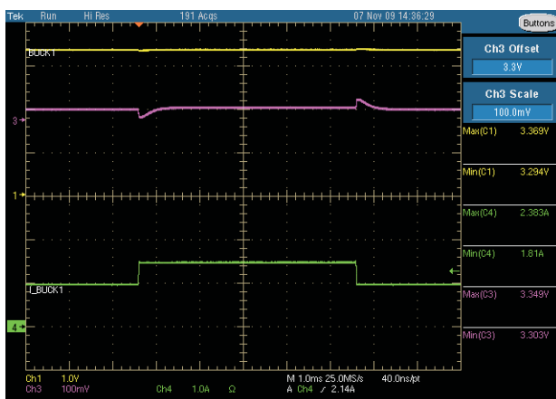
Figure 9. Transient Load Response V_{OUT} = 3.3\text{ V} , \Delta I = 1\text{ A} to 1.5\text{ A} , 100\text{ mV/div}
