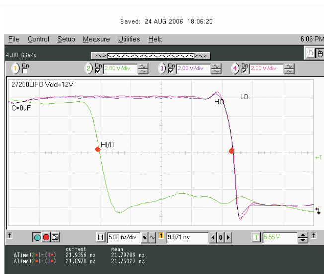
Figure 31. V_{LO} and V_{HO} Falling Edge Delay Matching
