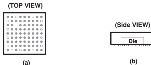
Figure 39. Views of Thermally-Enhanced GQE Package
