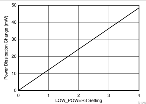
图 8-13. Power Dissipation Change vs LOW_POWER3 register setting
