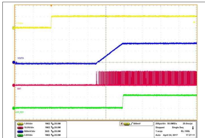
V_{VIN} = 12\text{ V} I_{OUTA} = 10\text{ A} V_{VOUT\_A} = 0.9\text{ V}
