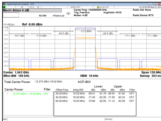
图 170. Dual band ACPR Performance in Downlink Band 3 with On-chip PLL
