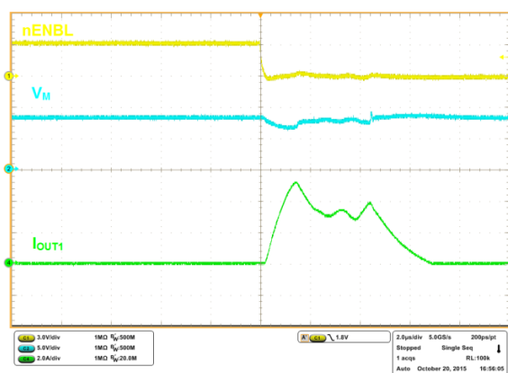
Figure 8. Current Ramp With a 16- \Omega , 1-mH, R_L Load and V_M = 8.2 V
