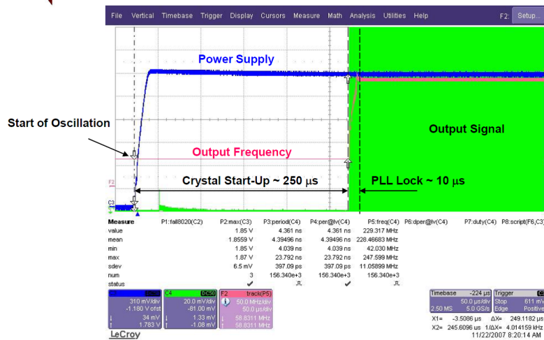
Figure 17. Crystal Oscillator Start-Up vs PLL Lock Time
