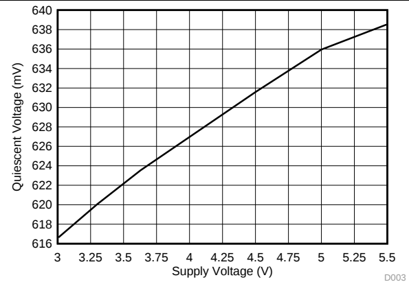
图 2. Quiescent Voltage vs Supply Voltage
