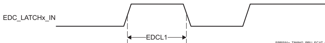
图 5-69. PRU-ICSS ECAT LATCHx_IN Timing
