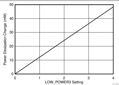
图 8-13. Power Dissipation Change vs LOW_POWER3 register setting
