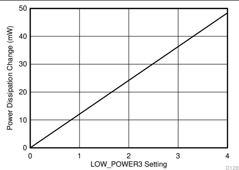
图 8-13. Power Dissipation Change vs LOW_POWER3 register setting
