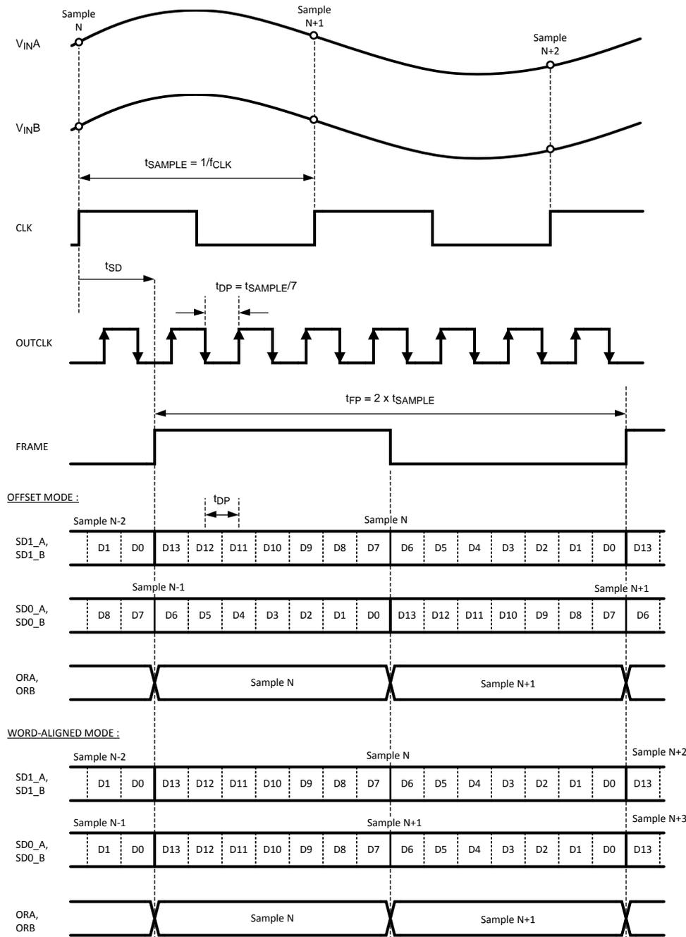
Figure 3. Serial Output Data Format in Dual-Lane Mode
