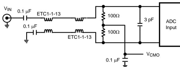
**Figure 20. High Input Frequency Transformer Drive Circuit**
