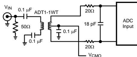
**Figure 19. Low Input Frequency Transformer Drive Circuit**
