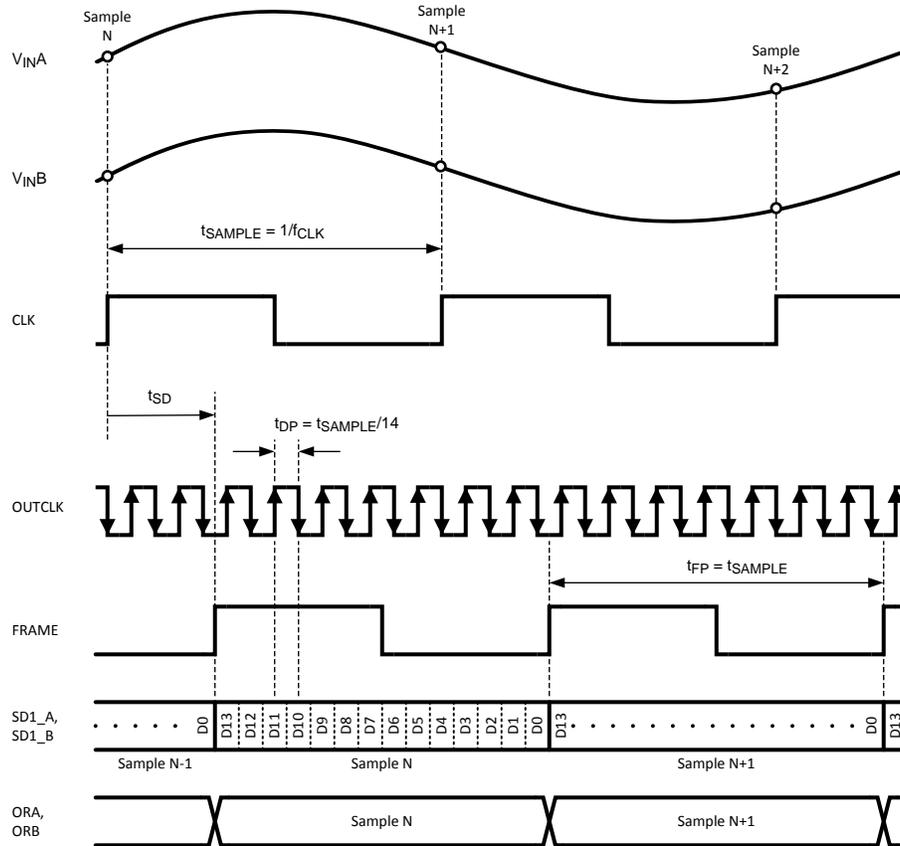
**Figure 2. Serial Output Data Format in Single-Lane Mode**
