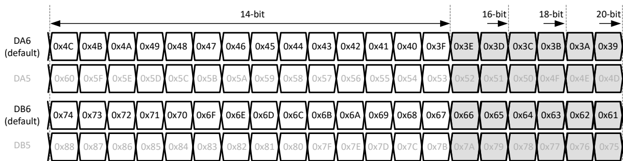
图 8-41. 1-wire output bit mapping
