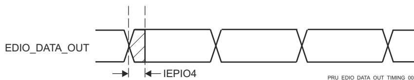
Figure 7-111. PRU_ICSSM IEP Digital IOs Timing Requirements
