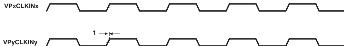
Figure 6-31. Video Port Dual-Display Sync Timing
