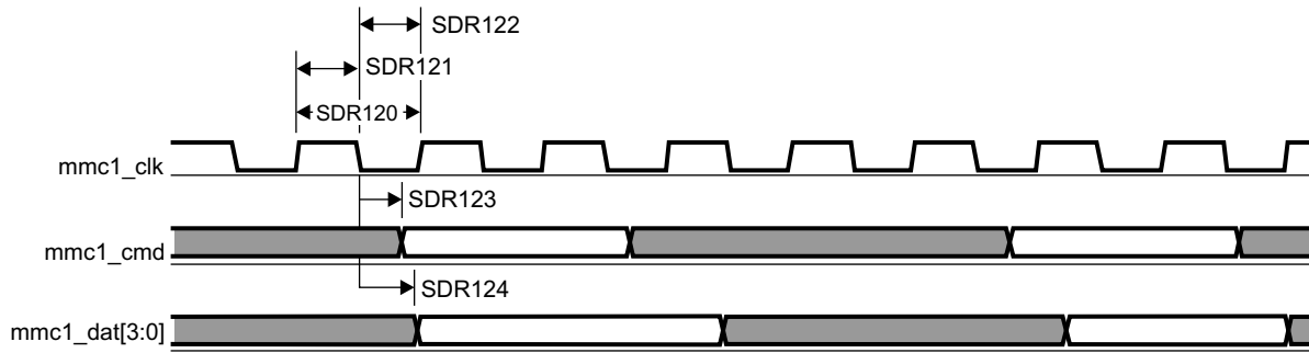
图 5-78. MMC/SD/SDIO in - High Speed SDR12 - Transmitter Mode
