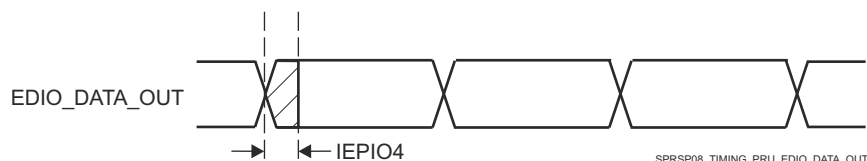
图 7-106. PRU_ICSSG PRU IEP Digital IOs Timing
