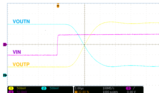
图 8-4. Step Response of the AMC1302
