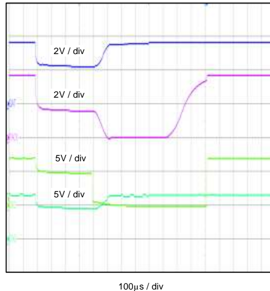
Figure 25. Short-Circuit in Discharge Protection Set and Clear
