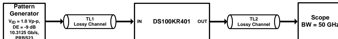
Figure 13. Test Setup Connections Diagram
