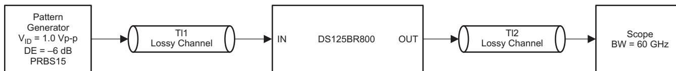
Figure 11. Test Setup Connections Diagram
